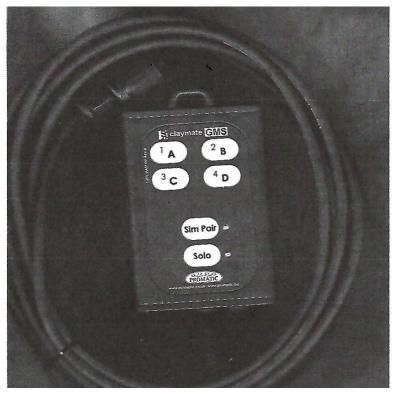
1. The picture above is of the handset controller on each station. The buttons "A,B,C & D" correspond to the target machines on the stations. The "Sim Pair" button is used when the menu reads TRUE PAIR.
